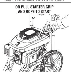
If the engine does not start after each pull of the starter grip and rope or after the engine switch is moved to the START position, squeeze the trigger to relieve water pressure before attempting to start the engine again.
