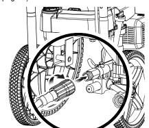
Completely uncoil and straighten high pressure hose to prevent kinks.
