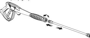
Connect the high pressure hose to the trigger handle
