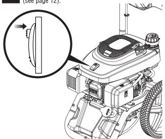
Slide the lock button down and push the engine switch to the START position. Engine can also be started by pulling the recoil starting grip until the engine runs (see page 12).
